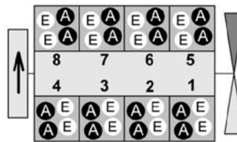
Fig. 5-22 Arrangement of cylinders, intake and exhaust valves
