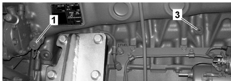
Fig. 5-29 Coolant draining valve and screw on engine front side
